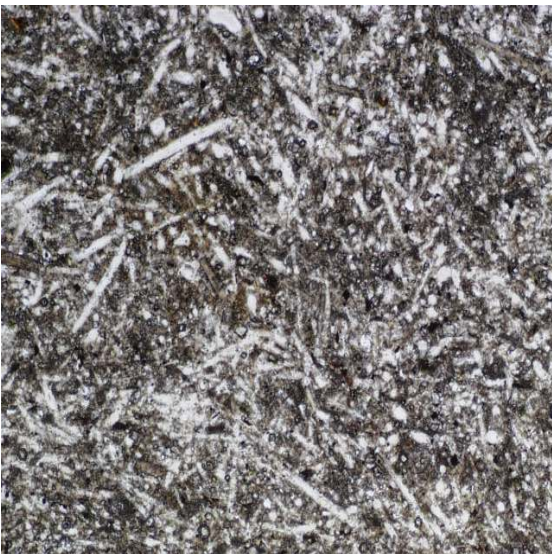
Figure 4. Thin-section micrograph of bedded Cowley spiculite. Woolsey “A” #5 Oakes, 4936', Barber Co., KS. Plane light, 40x magnification.
